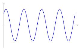
**No Damping**: Solution oscillates with natural frequency (here  $\omega_0 = 4$ )
