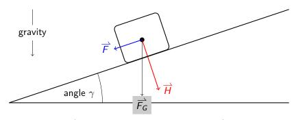
Can compute  $\overrightarrow{F}_G$  from the weight but we want:  $\overrightarrow{F}$ , the force acting on the block in the direction of the slope.
