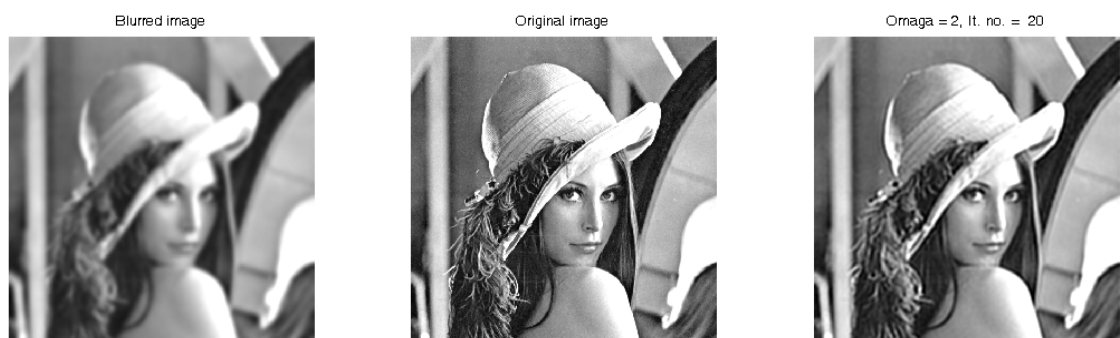
Figure 24: Original image (center), blurred image to the left, and deconvolved image ( \omega = 2 , 20 iterations) to the right.
