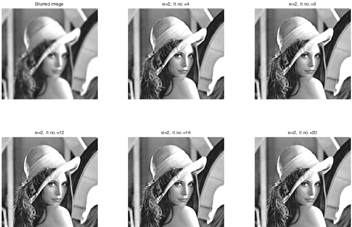
Figure 22: Van Cittert deconvolution applied to a blurred version of Lena .
