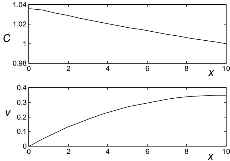
**Figure 19:** Solution obtained with the "shooting method". Parameter values:  $\lambda = 10$ ,  $\kappa = 1$ ,  $\varepsilon = .5$ . In order to end in 1 for  $x = 10$ ,  $C(0)$  must be about 1.0355.
