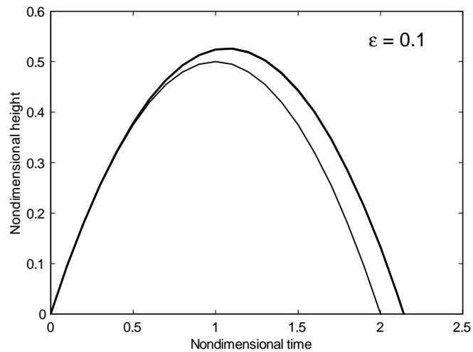
**Figure 12:** Numerical solution and perturbation solutions for  $\varepsilon = 0.1$ . The numerical solution (thick line) and the perturbation solutions to first and second order collapse on the graph. The solution for  $x_1$  is different, however.
