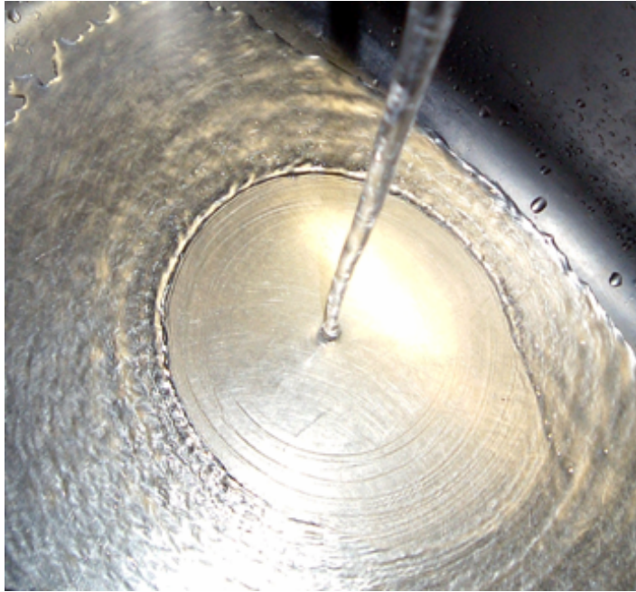
Figure 23: When a vertical water stream hits a horizontal surface, a circular jump in the flow forms some distance away from where the stream hits.
