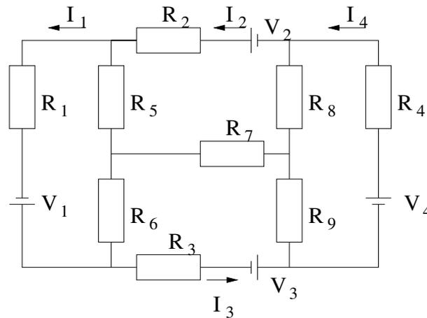
We would like to find the currents  $I_i$ ,  $i = 1, \dots, 4$  when the resistances  $R_i$ ,  $i = 1, \dots, 9$  and the voltage sources  $V_i$ ,  $i = 1, \dots, 4$  are given. Kirshoffs laws together with Ohm's law gives the following system of equations:
