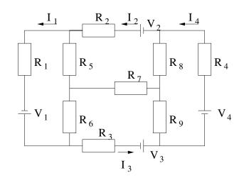
We would like to find the currents  $I_i$ , i = 1, ..., 4 when the resistances  $R_i$ , i = 1, ..., 9 and the voltage sources  $V_i$ , i = 1, ..., 4 are given. Kirshoffs laws together with Ohm's law gives the following system of equations:
