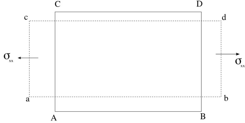
Figure 5: Deformed geometry under axial stresses
