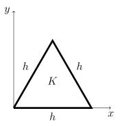
**b)** Find the three linear shape functions for the element K. Find the elemental stiffness matrix  $A^{K}$  and the elemental load vector  $\mathbf{b}^{K}$ .
