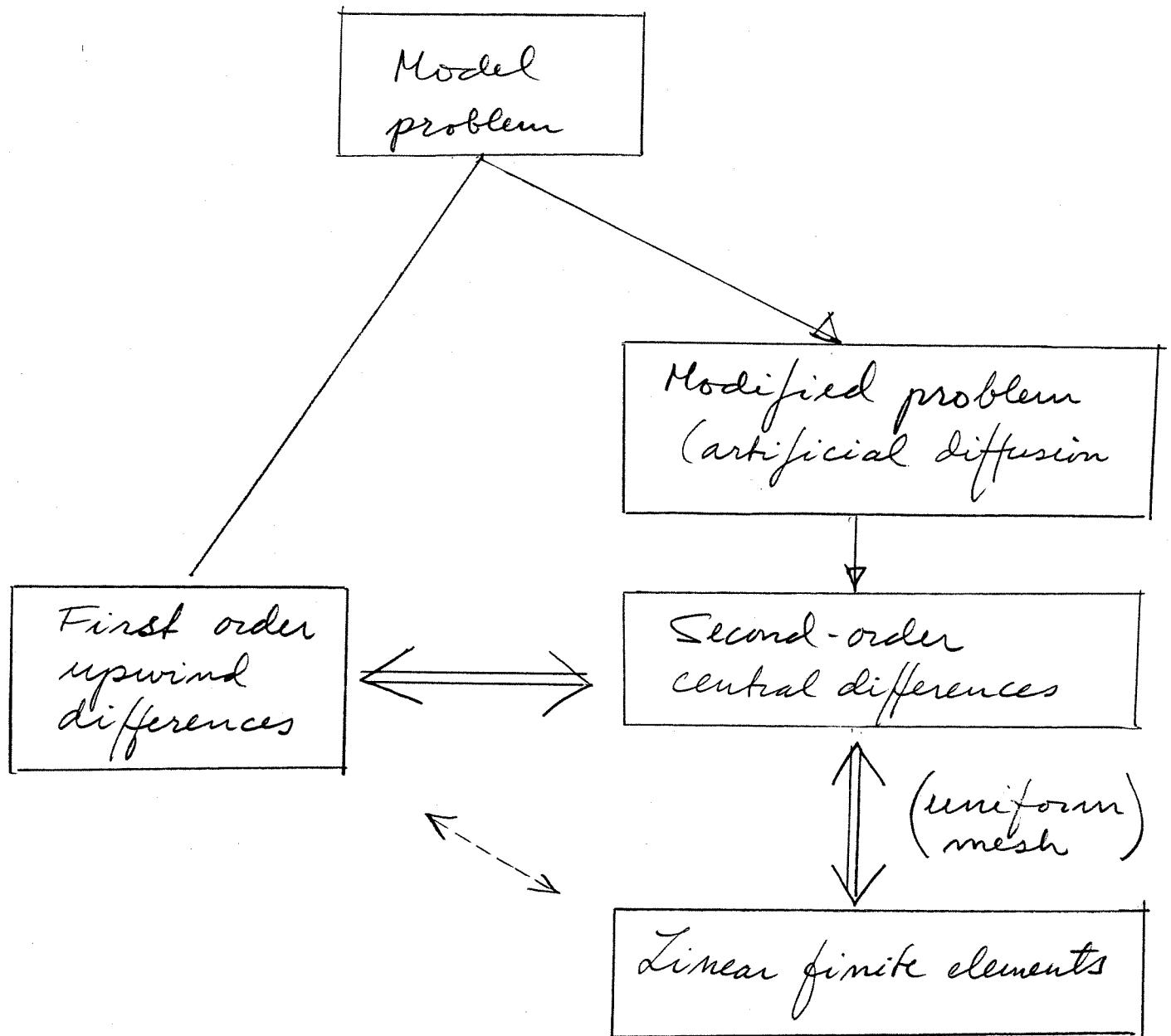
Hence, in the finite element context, we can include the effect of upwinding by discretizing a modified problem where we have added a proper amount of artificial diffusion.
