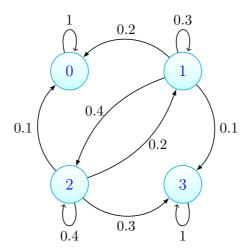
The state 0 does not communicate with any other state and hence forms one equivalence class. States 1 and 2 communicate and build a second equivalence class, and state 3 forms a third equivalence class as it does not communicate with any other state.
