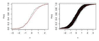
(Left: Estimation of CDF from a normal sample of 100 points, Right: Variation of the estimation over 200 samples.)
