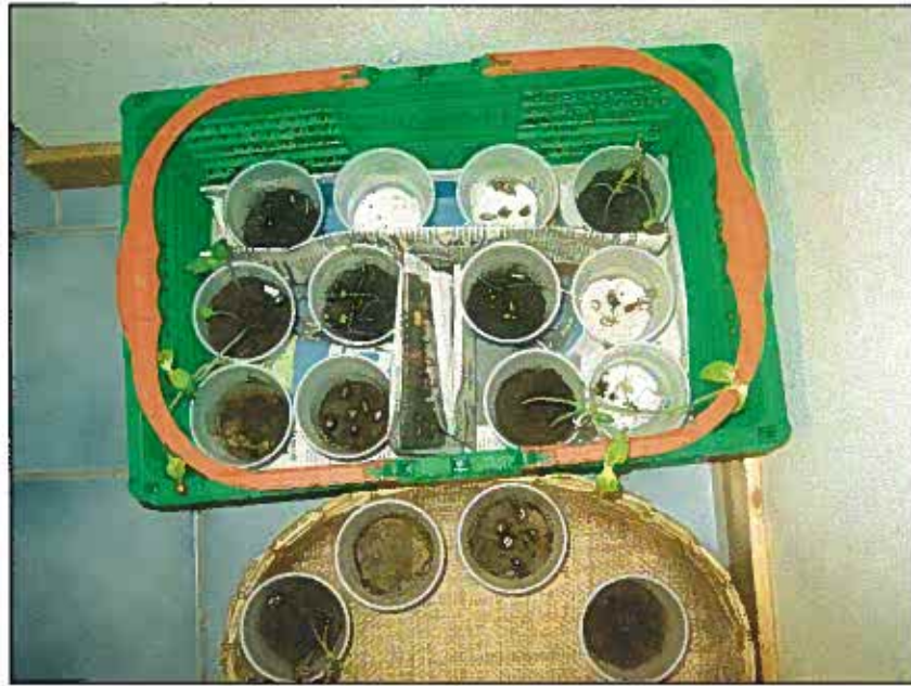
Figure 1.1 Box and 16 containers with the seeds: during the experience all the glasses were put inside the green box which was covered with a plastic film on the top to guarantee proper humidity conditions.
