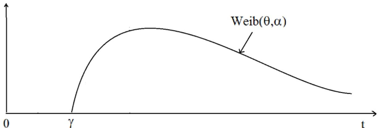
$$\begin{aligned}f(t; \theta, \alpha, \gamma) &= \frac{\alpha}{\theta^\alpha} (t - \gamma)^{\alpha-1} e^{-(\frac{t-\gamma}{\theta})^\alpha}; & t > \gamma \\&= 0 \quad \text{otherwise}\end{aligned}$$
