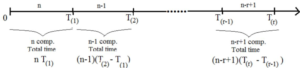
$n$  units put on test at time  $t = 0$ . Stop after a given number  $r$  of failures.
