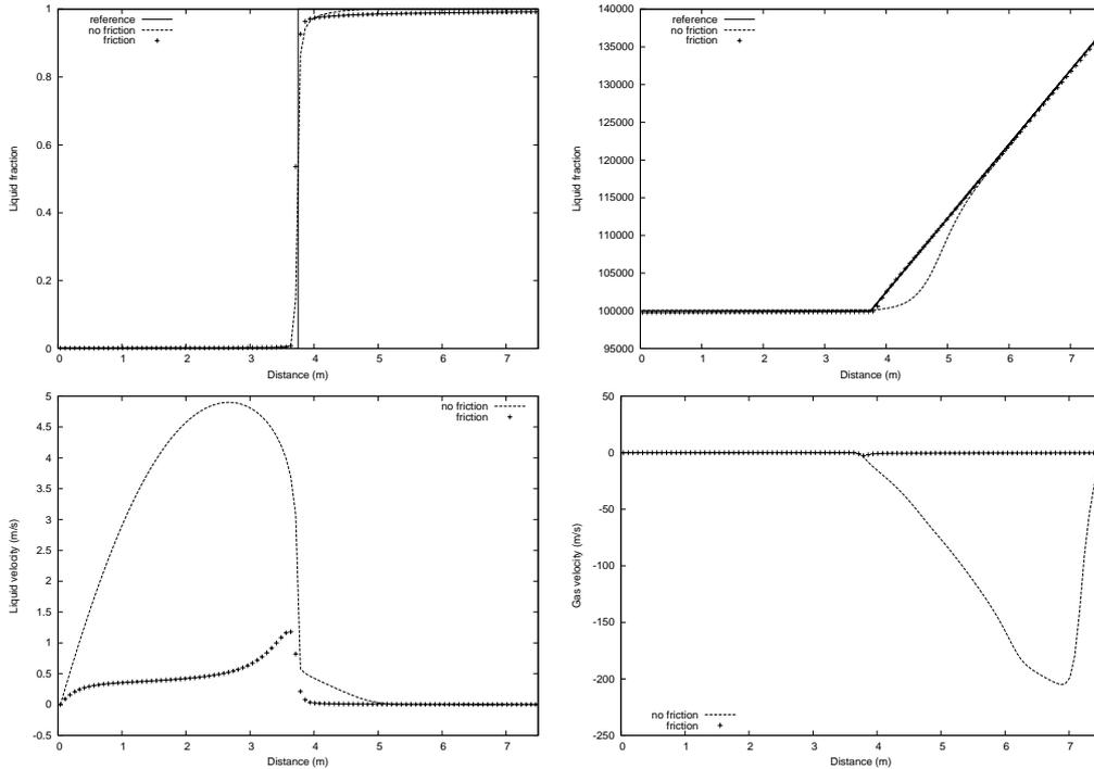
FIGURE 10. Separation problem,  $t = 5.0$  s, 100 grid cells. WIMF-AUSMDV\* scheme with and without interfacial momentum exchange terms. Top left: Liquid fraction. Top right: Pressure. Bottom left: Liquid velocity. Bottom right: Gas velocity.
