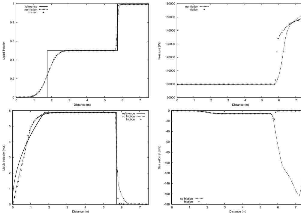
FIGURE 9. Separation problem,  $T=0.6$  s, 100 grid cells. WIMF-AUSMDV\* scheme with and without interfacial momentum exchange terms. Top left: Liquid fraction. Top right: Pressure. Bottom left: Liquid velocity. Bottom right: Gas velocity
