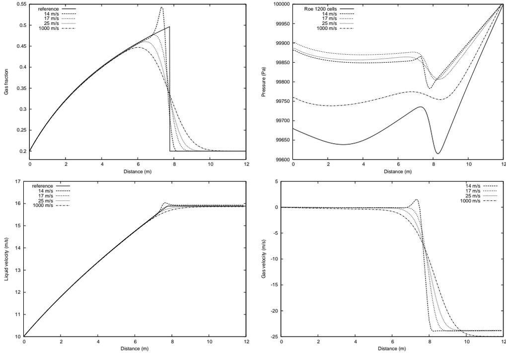
FIGURE 6. Water faucet problem, 120 cells,  $T=0.6$  s. Different timesteps for the WIMF-AUSMD scheme. Top left: Gas fraction. Top right: Pressure. Bottom left: Liquid velocity. Bottom right: Gas velocity.
