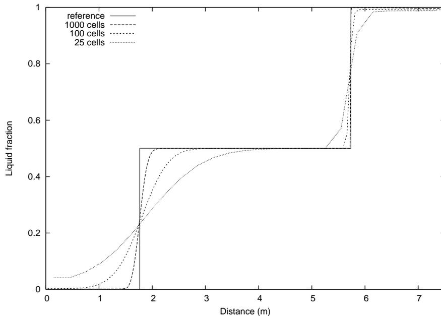
FIGURE 11. Separation problem,  $T=0.6$ s. Convergence properties of the WIMF-AUSMDV\* scheme with interfacial momentum exchange terms.
