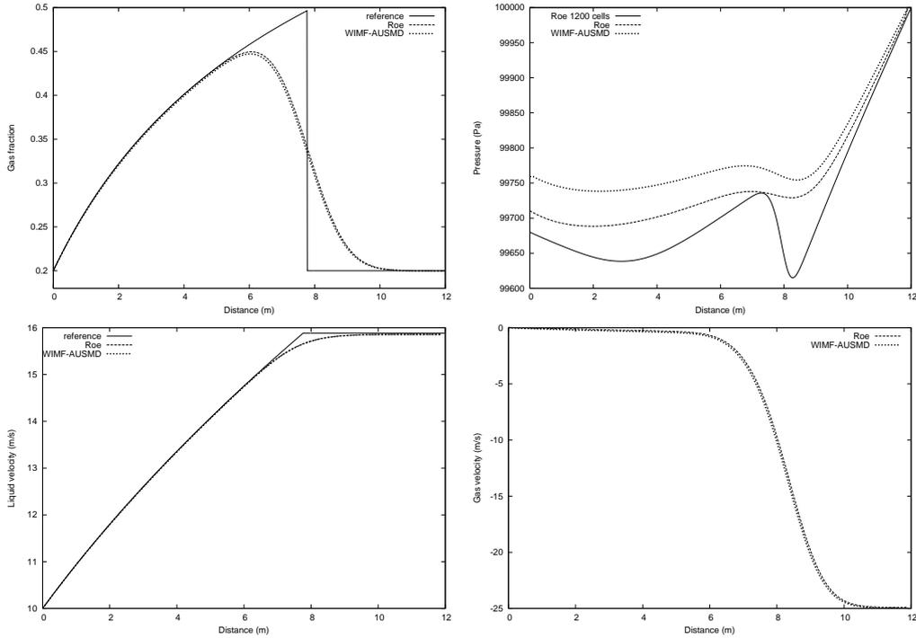
FIGURE 5. Water faucet problem, 120 cells,  $T=0.6$  s. Roe vs WIMF-AUSMD,  $\Delta x/\Delta t = 10^3$  m/s. Top left: Gas fraction. Top right: Pressure. Bottom left: Liquid velocity. Bottom right: Gas velocity.
