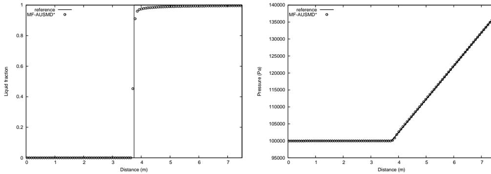
FIGURE 14. Separation problem,  $T=1.5$  s. MF-AUSMD\* scheme, 100 cells. Top left: Liquid fraction. Top right: Pressure. Bottom left: Liquid velocity. Bottom right: Gas velocity.
