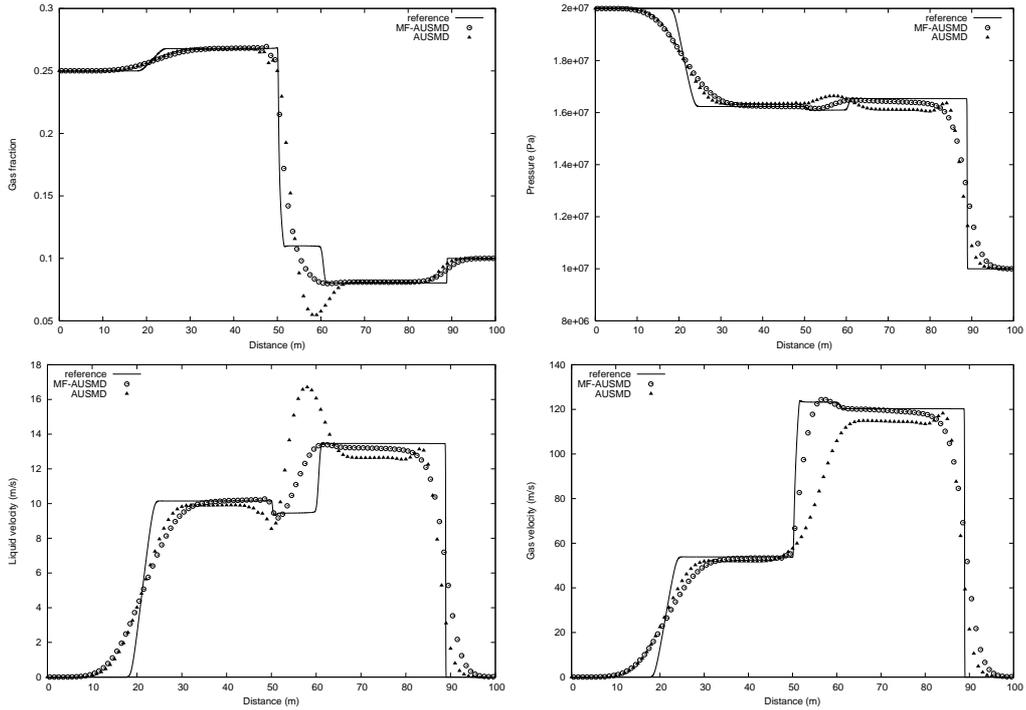
FIGURE 7. Toumi's shock tube problem,  $T = 0.08$  s, 100 grid cells. MF-AUSMD vs basic AUSMD scheme. Top left: Gas fraction. Top right: Pressure. Bottom left: Liquid velocity: Bottom right: Gas velocity.
