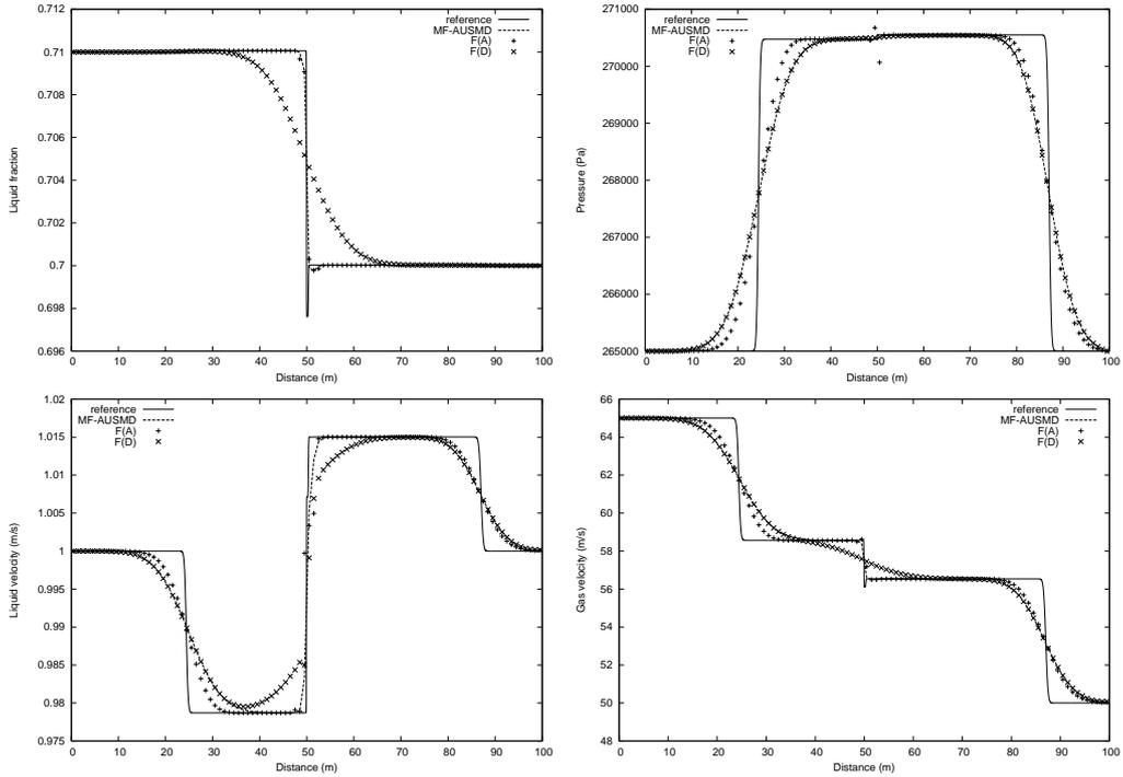
FIGURE 4. LRV shock tube problem,  $T = 0.1$  s, 100 grid cells. MF-AUSMD vs the purely diffusive ( $F_k^D$ ) and accurate ( $F_k^A$ ) components. Top left: Liquid fraction. Top right: Pressure. Bottom left: Liquid velocity: Bottom right: Gas velocity.
