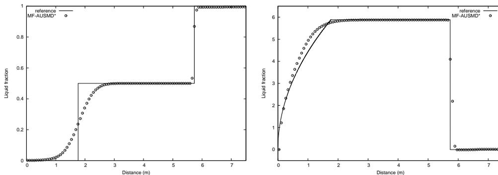
FIGURE 13. Separation problem,  $T=0.6$  s. MF-AUSMD\* scheme, 100 cells. Left: Liquid fraction. Right: Liquid velocity.
