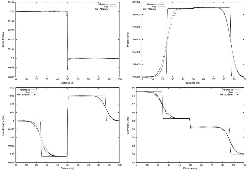
FIGURE 3. LRV shock tube problem,  $T = 0.1$  s, 100 grid cells. MF-AUSMD vs Roe scheme. Top left: Liquid fraction. Top right: Pressure. Bottom left: Liquid velocity: Bottom right: Gas velocity.
