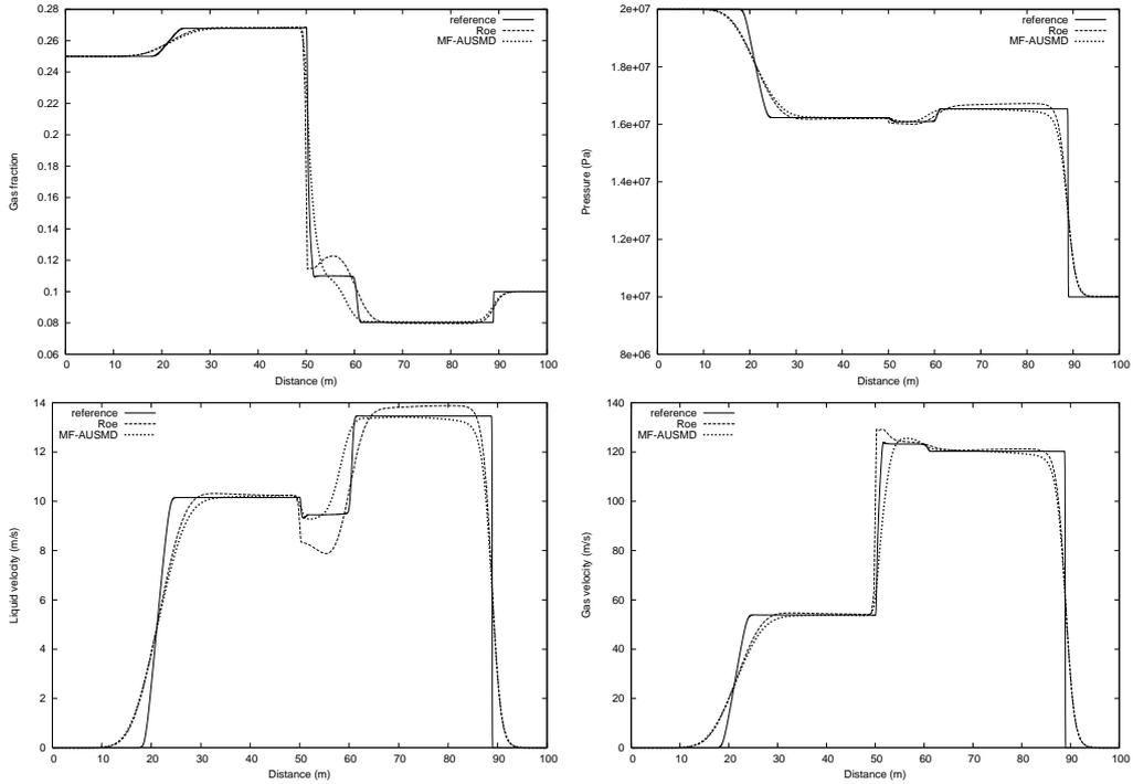
FIGURE 8. Toumi's shock tube problem,  $T = 0.08$ , 200 grid cells. MF-AUSMD vs Roe scheme. Top left: Gas fraction. Top right: Pressure. Bottom left: Liquid velocity; Bottom right: Gas velocity.
