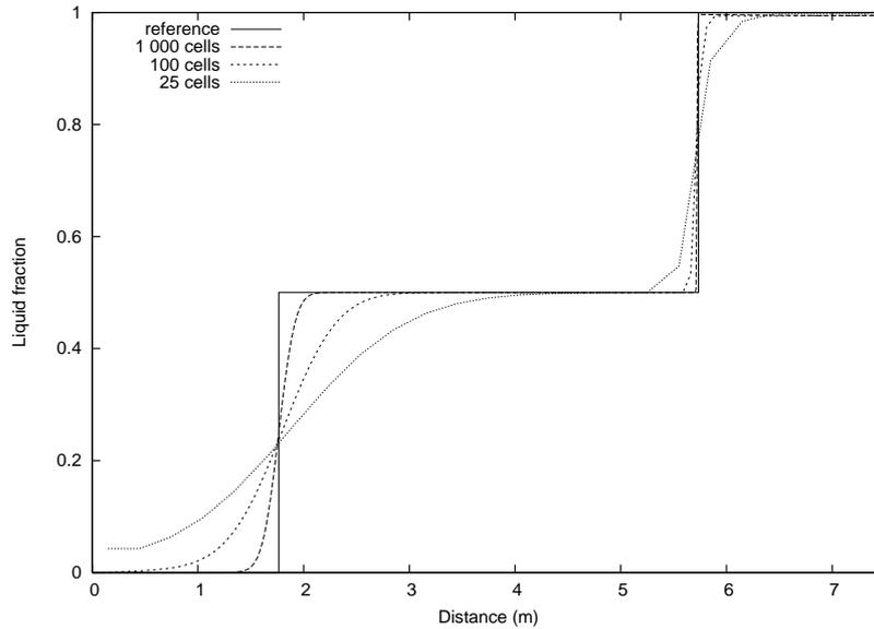
FIGURE 15. Separation problem,  $T=0.6$ s. Convergence properties of the MF-AUSMD\* scheme.
