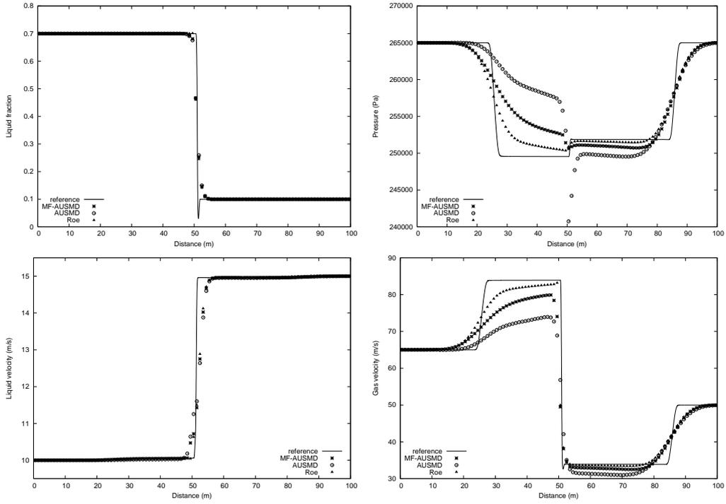
FIGURE 6. Modified LRV shock tube problem,  $T = 0.1$  s, 100 grid cells. MF-AUSMD, AUSMD and Roe scheme. Top left: Gas fraction. Top right: Pressure. Bottom left: Liquid velocity: Bottom right: Gas velocity.
