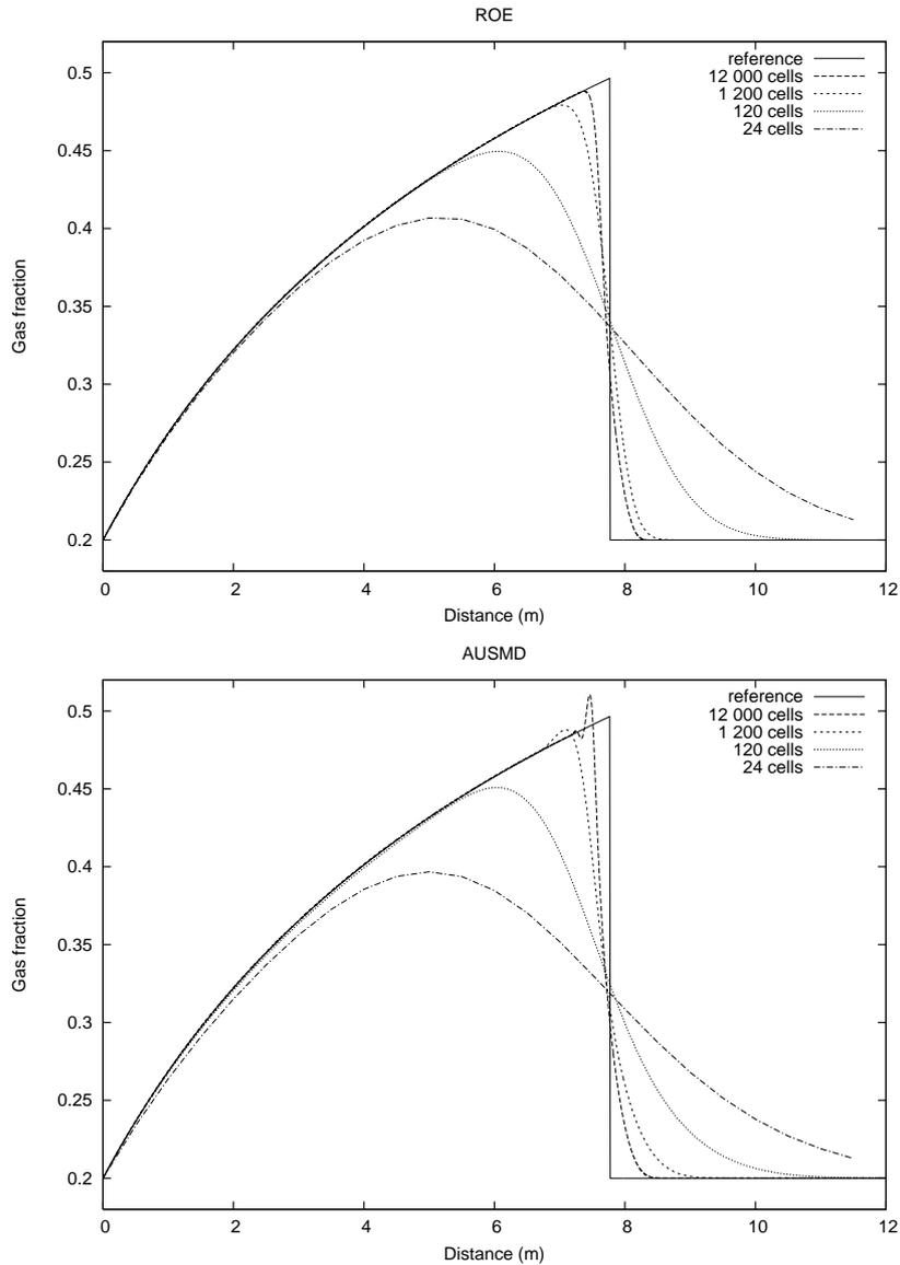
FIGURE 2. Water Faucet.  $t=0.6$  s. Accuracy on volume fraction. Top: Grid refinement for Roe scheme. Bottom: Grid refinement for AUSMD scheme.
