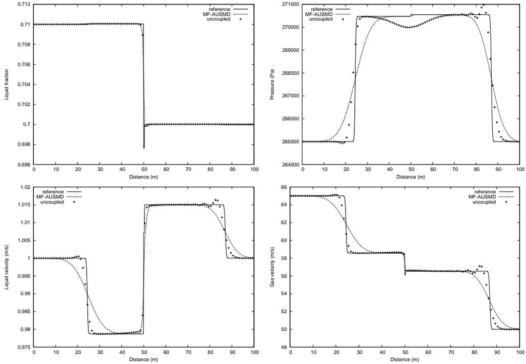
FIGURE 5. LRV shock tube problem,  $T = 0.1$  s, 100 grid cells. Lax-Friedrichs based MF-AUSMD vs FTCS based MF-AUSMD. Top left: Liquid fraction. Top right: Pressure. Bottom left: Liquid velocity; Bottom right: Gas velocity.
