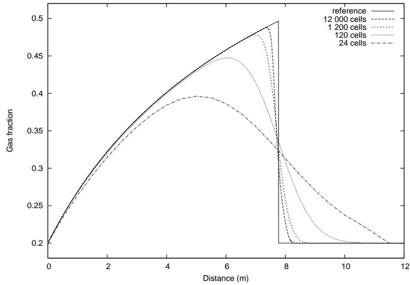
FIGURE 11. Water faucet problem,  $T=0.6$  s. Convergence properties of the MF-AUSMD scheme.
