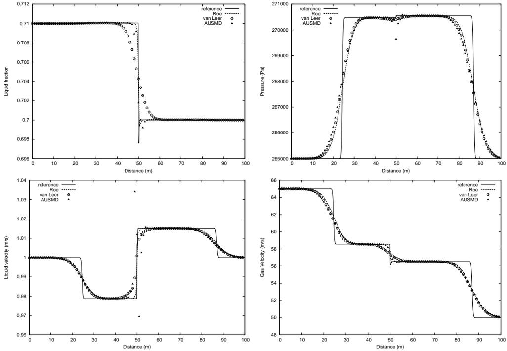
FIGURE 1. LRV shock tube problem. Comparison between van Leer, AUSMD, and Roe scheme on a grid of 100 cells. Top left: liquid fraction. Top right: pressure. Bottom left: liquid velocity. Bottom right: gas velocity.
