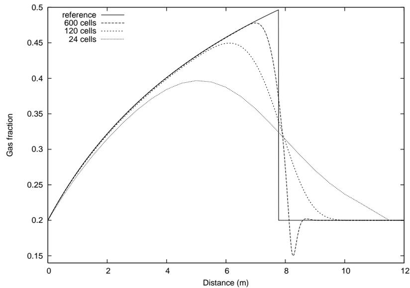
FIGURE 12. Water faucet problem,  $T=0.6$ s. Non-hyperbolic model. Convergence properties of the MF-AUSMD scheme.
