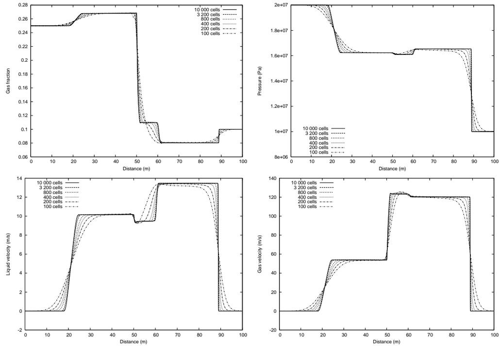
FIGURE 9. Toumi's shock tube problem. Grid refinement for the MF-AUSMD scheme. Top left: Gas fraction. Top right: Pressure. Bottom left: Liquid velocity; Bottom right: Gas velocity.
