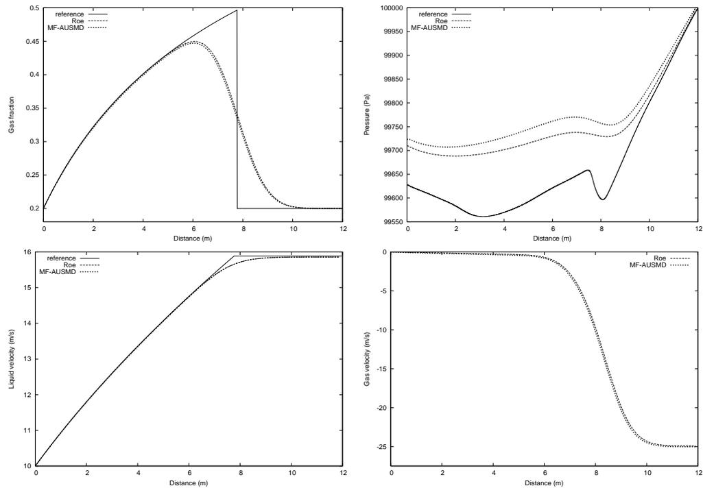
FIGURE 10. Water faucet problem,  $T = 0.6$  s, 120 grid cells. MF-AUSMD vs Roe scheme. Top left: Gas fraction. Top right: Pressure. Bottom left: Liquid velocity; Bottom right: Gas velocity.
