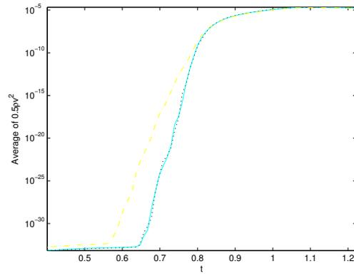
FIGURE 3.14. Logarithm of average  $\frac{1}{2}\rho v^2$  vs. time  $t$ . We see data from PPM as a dotted line, PPM-HLLC solid blue and RK-HLLC dashed yellow. The resolution was  $\Delta x = \Delta y = 0.02$ .
