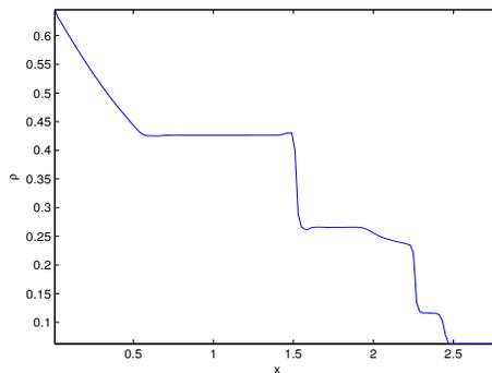
FIGURE 3.12. Slice of Richtmeyer-Meshkov instability at  $t = 1$ ,  $y = 0.49$ , Computed with PPM at resolution  $\Delta x = \Delta y = 0.02$ .
