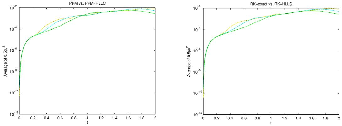
FIGURE 3.1. Growth of transversal kinetic energy component. The codes with exact solver are represented with dotted lines, and the HLLC version with solid coloured lines, green for  $100^2$  grid cells resolution, blue for  $200^2$  and yellow for  $400^2$  grid cells.
