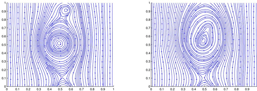
FIGURE 3.7. Streamlines from simulations with  $400^2$  cells at time  $t = 16$ . RK-HLLC is shown on the left, and RK-exact right.\*
