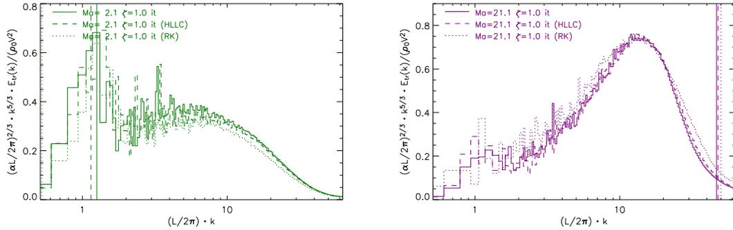
FIGURE 4.11. Compensated energy spectra for isentropic runs from the final time  $t = 5T$ . On the left  $Ma=2.1$ , and on the right  $Ma=21.1$ . The vertical lines represent the 'sonic wave number'. Integrating the curve to the left of this line gives  $c_s^2$ . The curves are labelled as in Figure 4.6.
