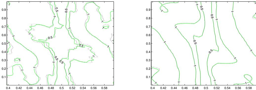
FIGURE 3.11. Superimposed density contours from Kelvin-Helmholtz instability with Mach number 10 at time  $t = 10$  at resolution  $200^2$  cells. On the left PPM is represented by green solid lines, and PPM-HLLC with dotted lines. On the right RK-exact with green solid lines, and RK-HLLC with dotted lines. RK right.\*
