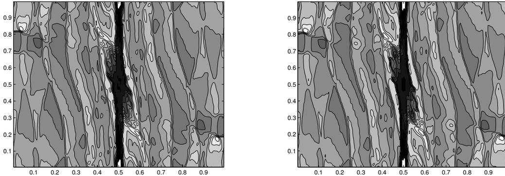
FIGURE 3.9. Density contours from Kelvin-Helmholtz instability with Mach number 10 at time  $t = 10$ . The resolution was  $200^2$  cells. PPM-HLLC is shown on the left, and PPM on the right. Density contours range from 0.4 to 1.4.\*
