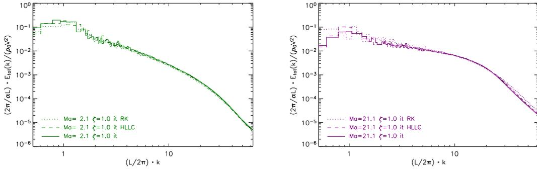
FIGURE 4.10. Energy spectra for isentropic runs from the final time  $t = 5T$ . On the left  $Ma=2.1$ , and on the right  $Ma=21.1$ . The curves are labelled as in Figure 4.6.
