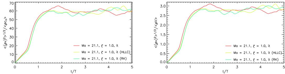
FIGURE 4.7. Time history of RMS (root mean squared) Mach number and momentum for isothermal run with characteristic Mach number  $Ma = 21.1$ . The curves are labelled as in Figure 4.6.
