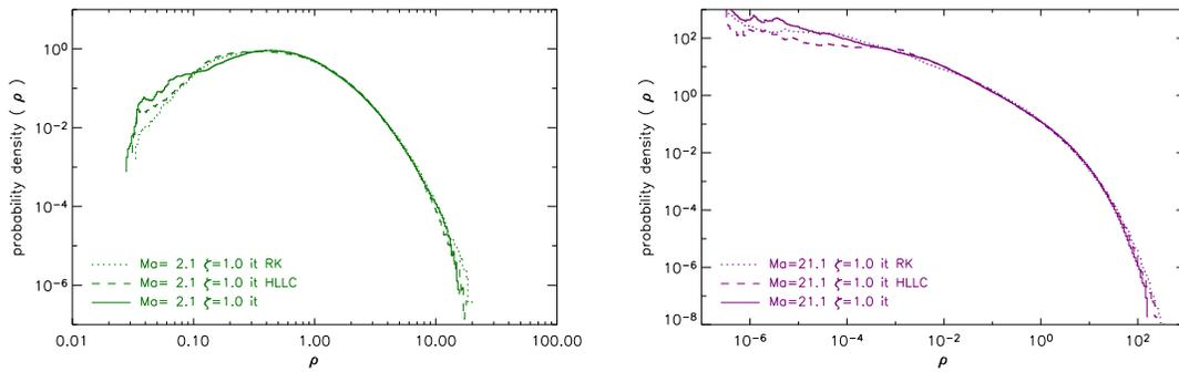
FIGURE 4.8. Density PDFs for isentropic runs from the final time  $t = 5T$ . On the left  $Ma = 2.1$ , and on the right  $Ma = 21.1$ . The curves are labelled as in Figure 4.6.
