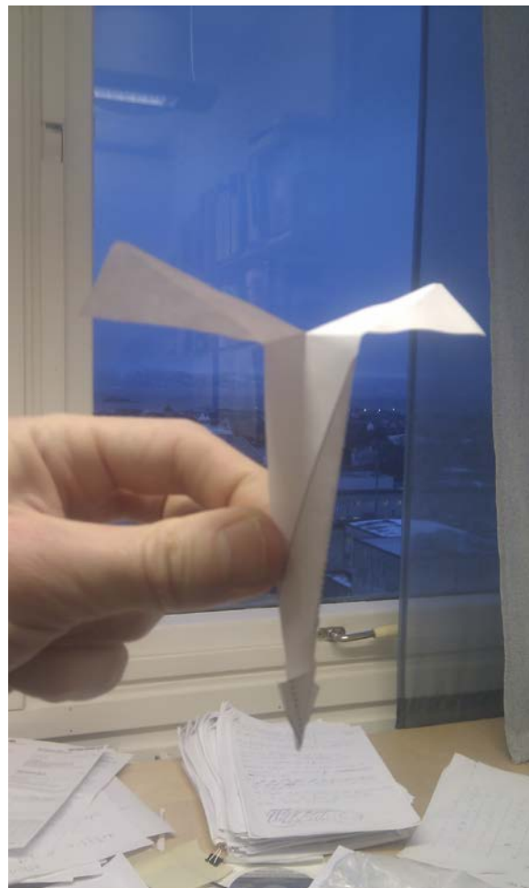
Figure 1: A “small” helicopter without a paper clip and with wings folded “down”.
