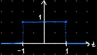
$$\begin{aligned}\hat{x}(\omega) &= \mathcal{F}(x(t)) = \frac{1}{2\pi} \int_{-\infty}^{\infty} x(t) e^{-i\omega t} dt = \frac{1}{2\pi} \int_{-1}^1 1 \cdot e^{-i\omega t} dt \\ &= \frac{1}{2\pi} \left[ \frac{1}{-i\omega} e^{-i\omega t} \right]_{-1}^1 = \frac{1}{-2\pi i\omega} (e^{-i\omega} - e^{i\omega}) = \frac{1}{\pi\omega} \cdot \frac{e^{i\omega} - e^{-i\omega}}{2i} = \underline{\underline{\frac{\sin(\omega)}{\pi\omega}}}\end{aligned}$$
