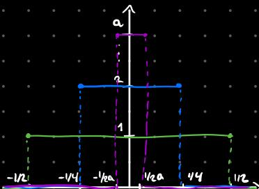
$$\hat{f}(\omega) = \mathcal{F}(f(t)) = \frac{1}{2\pi} \int_{-\infty}^{\infty} f(t) e^{-i\omega t} dt = \frac{1}{2\pi} \int_{-1/2a}^{1/2a} a e^{-i\omega t} dt = \frac{1}{2\pi} \left[ \frac{a}{-i\omega} e^{-i\omega t} \right]_{-1/2a}^{1/2a}$$
