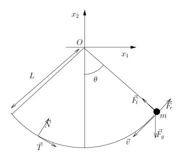
A pendulum of mass m and length L and point of fixation O is set in motion. The position  $\vec{x}$  of the pendulum is constrained to be on the circle
