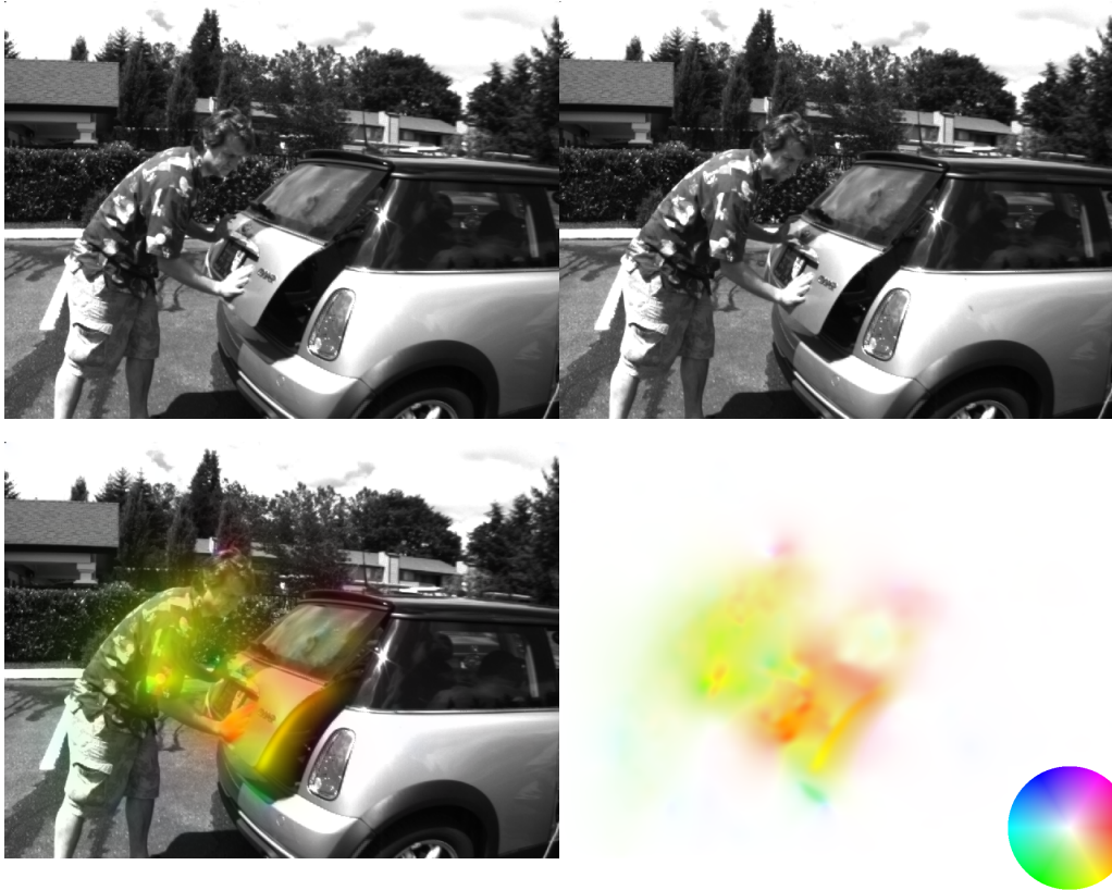
Figure 1: Result of an optical flow computation. First row: Two consecutive frames in an image sequence. Second row: The resulting flow ( right ) and the first frame of the sequence overlaid with the flow ( left ). The colourwheel on the bottom right indicates the direction and intensity of the flow field at each pixel. The test images have been taken from http://vision.middlebury.edu/flow/ .
