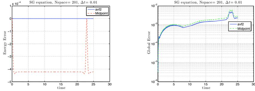
Figure 2.2: Sine-Gordon equation with spectral semi-discretization: Energy error (left) and global error (right) vs time, for AVF and implicit midpoint integrators.
