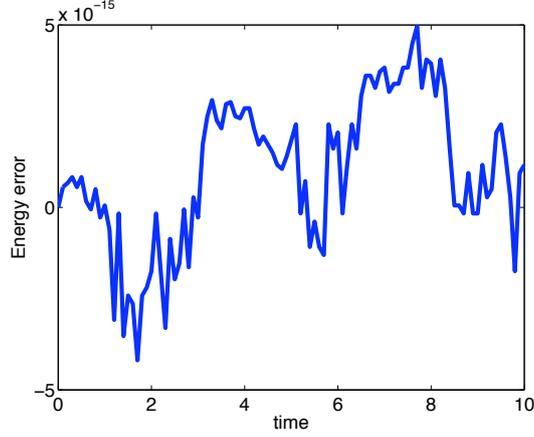
Figure 2.8: Linear Schrödinger equation: Error in energy  $\overline{\mathcal{H}}_1 \Delta x$  vs time, AVF method
