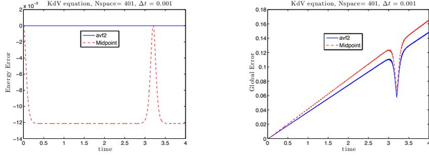
Figure 2.3: Korteweg-de Vries equation: Energy error (left) and global error (right) vs time, for AVF and implicit midpoint integrators.
