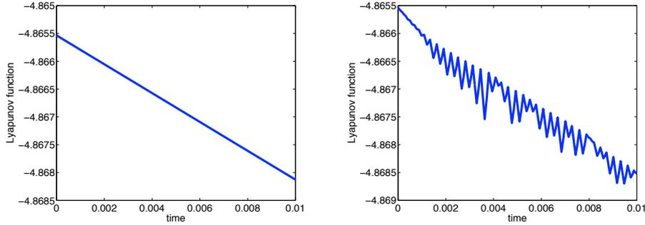
Figure 3.3: Ginzburg-Landau equation: Plots of the energy function  $\overline{\mathcal{H}}\Delta x$  computed with the AVF method (left) and Matlab's `ode45` (right). Note that `ode45` does not exhibit the correct monotonic decrease in energy.
