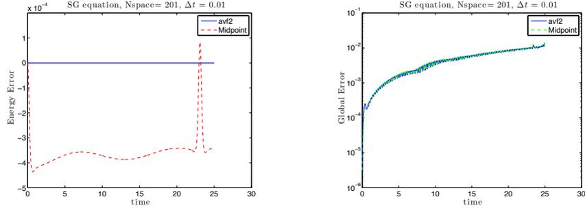
Figure 2.1: Sine-Gordon equation with finite differences semi-discretization: Energy error (left) and global error (right) vs time, for AVF and implicit midpoint integrators.
