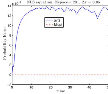
Figure 2.5: Nonlinear Schrödinger equation: Total probability error vs time, for AVF and implicit midpoint integrators.
