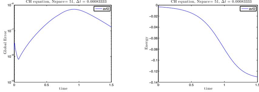
Figure 3.2: Cahn-Hilliard equation: Global error (left) and energy (right) vs time, AVF integrator.
