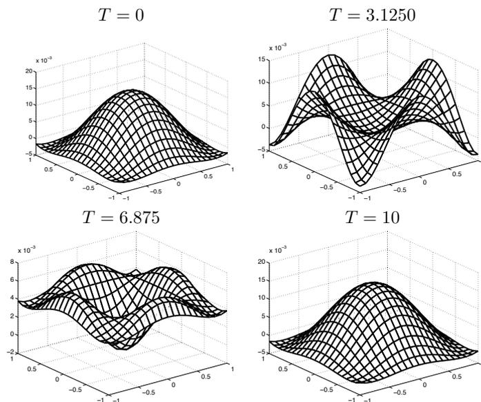
Figure 2.6: Snapshots of the solution of the 2D wave equation at different times. AVF method with step-size  $\Delta t = 0.6250$ . Space discretization with 6 Gauss Lobatto nodes in each space direction. Numerical solution interpolated on a equidistant grid of 21 nodes in each space direction.
