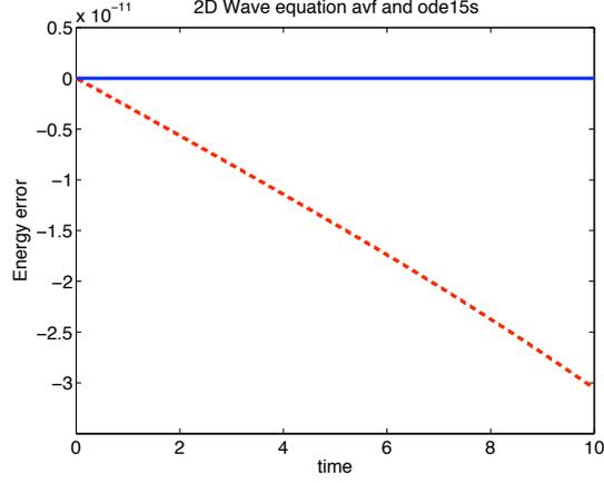
Figure 2.7: The 2D wave equation (2.25). MATLAB routine `ode15s` with absolute and relative tolerance  $10^{-14}$  (dashed line), and AVF method with step size  $\Delta t = 10/(2^5)$  (solid line). Energy error versus time. Time interval  $[0, 10]$ . Space discretization with 6 Gauss Lobatto nodes in each space direction.
