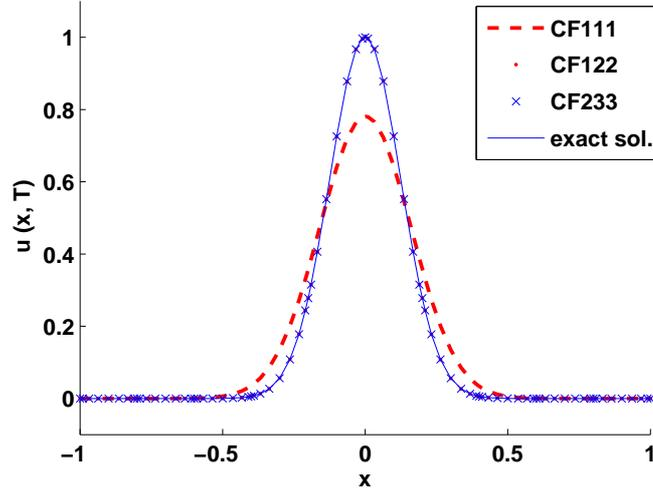
Figure 1: SLDG methods with  $p = 8, N_e = 10$  for Gauss cone advection in 1D, using first, second and third order time integrators CF111, CF122 and CF233. The exact solution is represent by the solid curve. The respective errors in the relative  $L_2$  norm are  $1.50 \times 10^{-1}, 2.00 \times 10^{-3}, 8.38 \times 10^{-6}$ . Meanwhile  $T = 1, n_{steps} = 400$  and  $C_r \approx 0.5$
