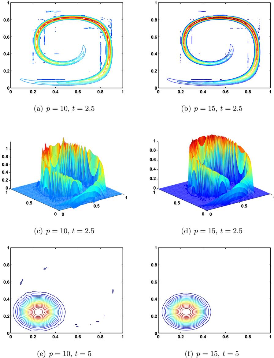
Figure 2: Tracer advection in 2D using CF233. In the first column,  $p = 10$ . In the second column,  $p = 15$ . The number of elements used in both case is  $N_e = 10 \times 10$ . First row: solution contours at  $t = 2.5$ ; Second row: solutions at  $t = 2.5$ ; third row: solution contours at  $t = 5$ . Contour levels:  $-36$  to  $36$  by  $18$ .
