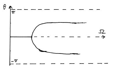
Figure 1: Bifurcation diagram for the bead on a rotating hoop
